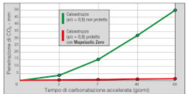
Fig. 2: Effect of Mapelastic Zero on accelerated carbonation (30% CO 2 ) in a porous concrete
